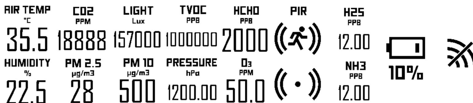
The information shown on the screen is based on user's choice of sensor. It would be refreshed by pressing the function key, triggering the PIR, or refreshed based on the report interval.
